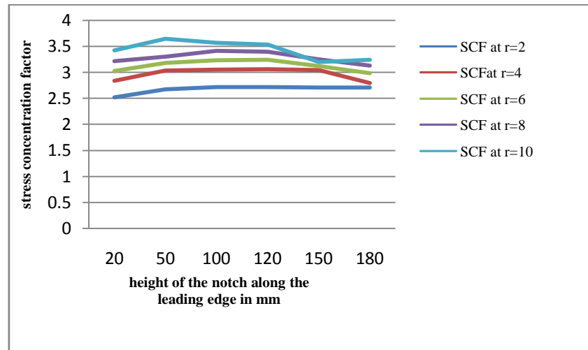
Graph.4 Stress concentration factor Vs height of the notch along the leading edge of the rectangular plate.
